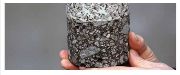
The Confalt Grouted Macadam system is an extremely hard wearing surface course with a high resistance to deformation, degradation and wear. Confalt can be installed onto almost any new or existing base, from cement stabilised gravel to asphalt, concrete and blocks.
